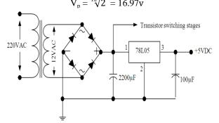
Figure 4: Circuit diagram for rectifying the power supply
